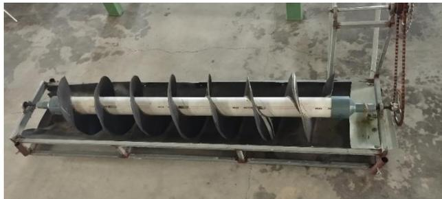
**Gambar 2.** Turbin Air Tipe *Screw* ARCHIMEDES
