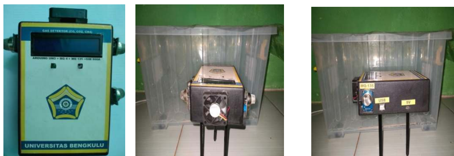
Figure 12. Implementation of CO, CO 2 , and CH 4 Gas Monitoring Equipment
